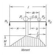
The maximum shear due to moving concentrated loads occurs at one support when one of the loads is at that support. With several moving loads, the location that will produce maximum shear must be determined by trial.
