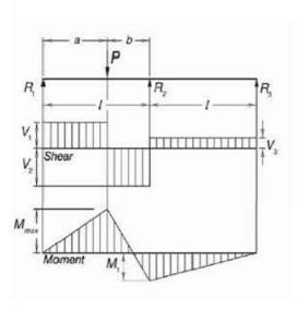
$$R_{1} = V_{1} \qquad \qquad = \frac{Pb}{4t^{3}} \left( 4t^{2} - a(t+a) \right)$$
