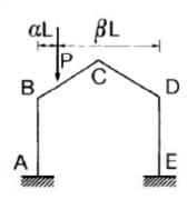
$$\begin{split} \chi_1 &= \frac{1}{K_2} \left[ 2\beta \ K_1 + 3\phi \ (2\alpha + K_1) - \phi^2 \ (1 + 4\alpha) \right. + \\ &- 4\alpha^2 \ \phi \ (2 + K_1) - 4 \ \alpha^2 \ \phi^2 \right] \end{split}$$
