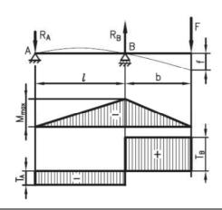
$$R_{A} = \frac{b}{l} \cdot F; \quad R_{B} = \frac{l+a}{l} \cdot F$$
