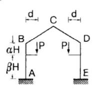
$$X_A = X_E = 6 \frac{Pd}{H} \frac{1}{K_2} [K_1 (1 + \varphi + \alpha) - \alpha (\alpha K_1 + \alpha + \varphi)]$$
