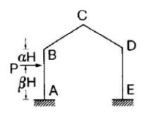
$$\begin{split} \chi_1 &= \frac{1}{K_2} \left[ K_1 \left( 4 + K_1 - 2\beta \ K_1 - 6\beta + 6 \ \phi \right) + \beta^2 \ K_1 \left( K_1 + 2 + \phi \right) + \right. \\ &\left. + 2\phi \ K_1 \left( 2\phi - \beta\phi - 3\beta \right) + \phi^2 \right] \end{split}$$
