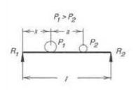
$$R_{1 \max} = V_{1 \max} (\text{at } x = 0)$$
