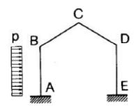
$$\chi_1 = \frac{1}{K_2} \left[ K_1 (6 + K_1) + K_1 \varphi (15 + 16\varphi) + 6 \varphi^2 \right]$$
